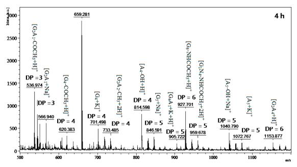
**Figure 7.** MALDI-TOF-MS of the oligomer mixtures obtained during water soluble chitosan hydrolysis. The proportion of low DP oligomer (DP < 7) was reduced by precipitation in the 90%methanol-soluble/90% acetone-insoluble fraction. The identified peaks are labeled with DP, in which DP indicates the degree of polymerization.
