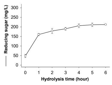
**Figure 6.** Hydrolysis time course measurement of reducing sugar with TKU029 chitosanase. The reaction mixture in a 250 mL Erlenmeyer flask containing 1% water soluble chitosan in 100 mL phosphate buffer (pH 7, 50 mM) and 10 mL of crude enzyme. The hydrolysis condition was carried at 50 °C in 6 h. The hydrolysis solution was then tested reducing sugar under the assay mentioned in the methods section. The error bars represent standard deviations (n = 3).
